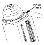
head assembly, simply unscrew the head lock ¼ turn and rotate it counter-clockwise.
