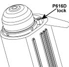
head assembly, simply unscrew the head lock 1/4 turn and rotate it counter-clockwise.
